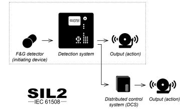
chain of devices necessary to detect and take appropriate action. A very simplified drawing showing a typical safety system for detection is shown below.
